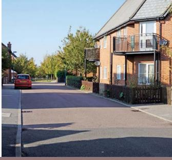
The access road is characterised by continuous asphalt surfaces, served by numerous road gulleys discharging directly to piped drainage.
