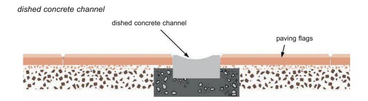
drainage channel with concrete haunching
