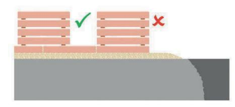
damaged flags can be kept for re-use as cut units
