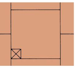
Where more than 25% of the flag has to be cut away then the remaining shape should be mitred from the internal corner of the cut-out to the external corner of the flag as shown below.
