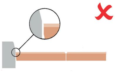
Cut faces should be positioned against an adjacent flag to reduce the visual intrusion of the square cut edge.
