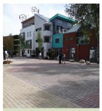
Concrete block permeable paving at the BRE Innovation Park.
