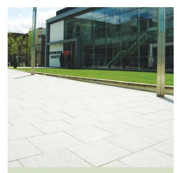
The latest products from Interpave manufacturers make use of the most sustainable resources while retaining impressive performance and visual characteristics. For example, here copper slag – a by-product from copper smelting – is used to create the decorative finish, while china clay stent – a by-product of the china clay industry – is used as an aggregate instead of quarrying virgin materials.
