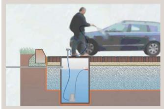
This is a more sustainable approach to car washing with most of the water automatically treated for reuse as it passes through the permeable paving.
