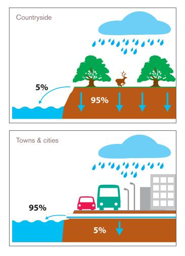
A lot of older sewers are known as 'combined sewers' carrying both rainwater and 'foul water' from toilets, baths, sinks, etc. They often have overflows that operate in heavy rain, diverting all the flows – including raw sewage – into rivers and streams, with serious consequences. As development increases and more rainwater runs into the sewers, the overflows are operating more often and therefore increasing pollution.
