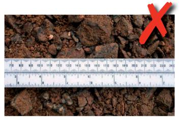
Type 1 aggregate for conventional block paving is not permeable when compacted.
