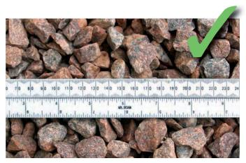
Typical permeable sub-base aggregate has voids between for water.
