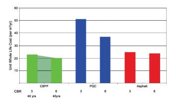
Estate Roads – Industrial – Initial costs for all types of CBPP are substantially lower than asphalt for CBR values of 4% or more, becoming similar for the lower values.
