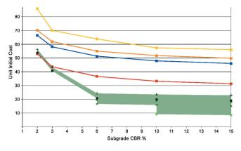
The loading regime on an industrial estate distribution road can be relatively severe, with a high proportion of heavy good vehicles. So, maintenance and WLCs are important, with CBPP (System C) offering the lowest WLC.
