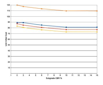
Airport Airside Pavements – considered from an initial cost perspective only. Costs of impermeable concrete block paving follow those for asphalt and are substantially lower than those for reinforced or PQ concrete until very low CBR values are reached.
