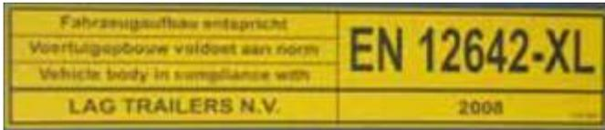
Trailer headboards which do not display this sticker do not meet the minimum requirements for XL rating.
