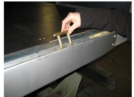
**Fig 3.** 'V groove' side rave lashing points are usually rated to 2,500 daN (kg), but some are only rated to 1,500 daN (kg); the rating is usually stamped on the lashing body. Check lashing for stamped rating.
